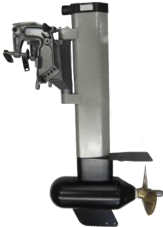
Figure: Outboarder with shaft-profile
